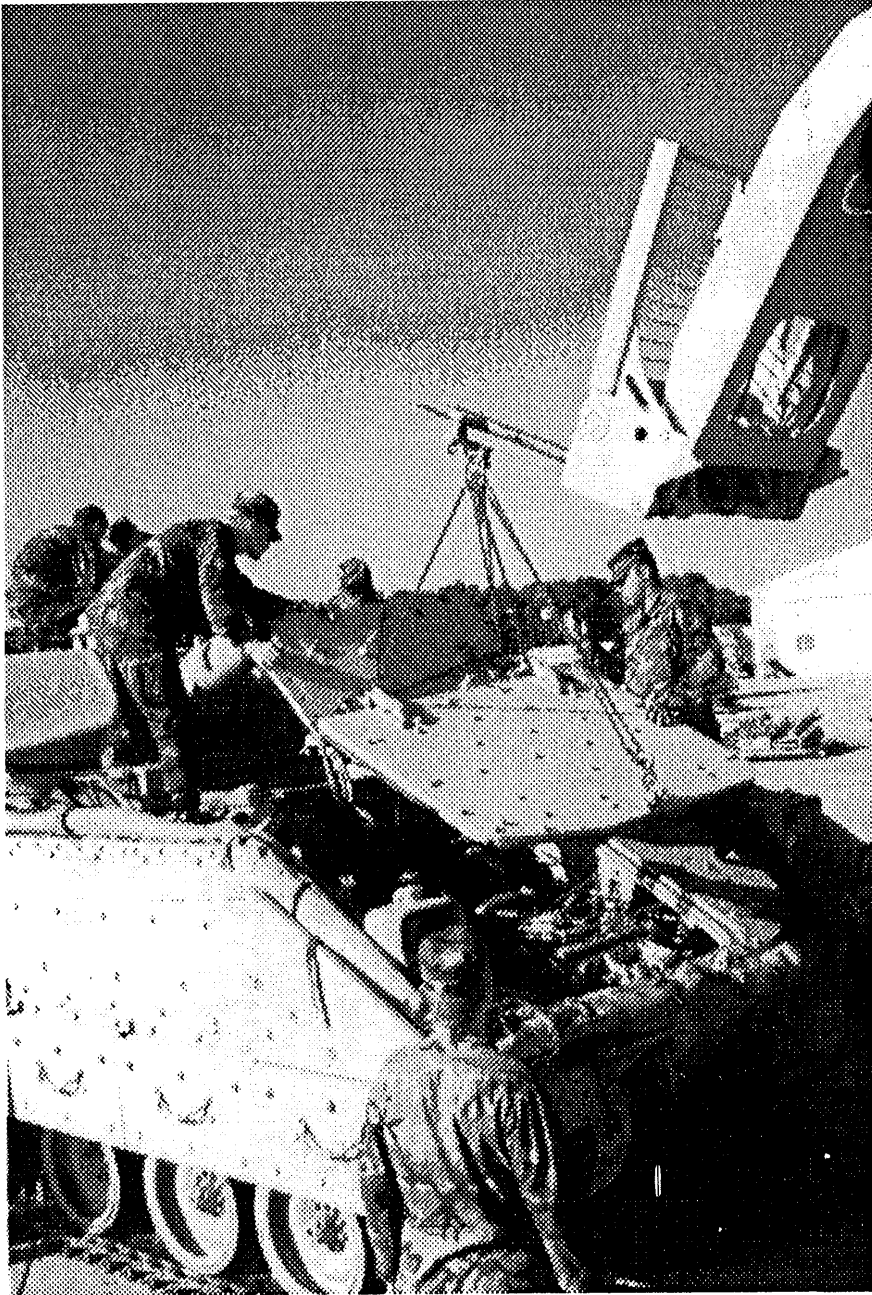
6,000 Pound forklift lowers engine access cover into place, guided by IRC platoon soldiers. The A-frame can also be used to perform this operation.
